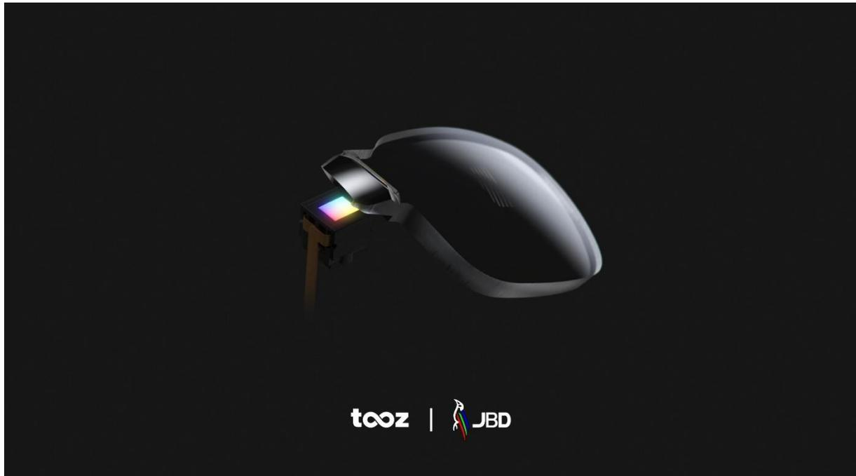
The curved waveguide by tooz and the color microLED display engine by JBD enable bright, full color virtual screens in the wearer's field of view. (© tooz technologies GmbH)
