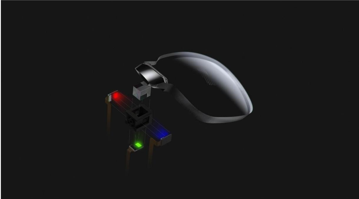
JBD and tooz combine a curved waveguide including prescription with a polychrome display engine consisting of a x-cube and a red, green and blue microLED display panel. (© tooz technologies GmbH)
